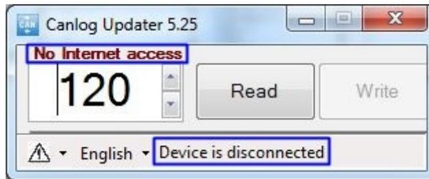
Figure 27. Internet and device connection errors
