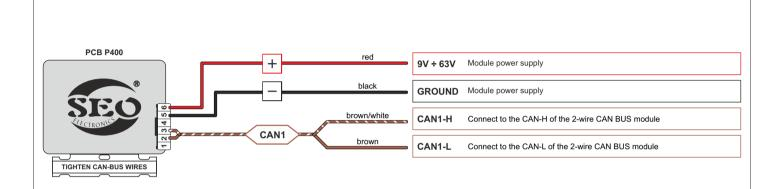
Contactless CAN BUS reader for any CAN BUS devices
